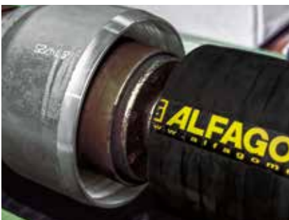
4. Coupling insertion on the hose
