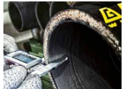
3. Hose thickness measurement is taken to identify the correct calibrated crimping diameter
